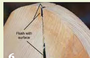
**6** Glue a half-pattern into the slot on each disk. The inside of each pattern should face the outside of the disk, away from the tenon. The trunk of the tree should be on the outside rim of the disk.
