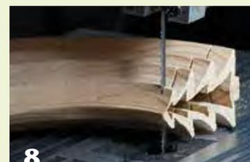
**8** With the outside profiles turned and the center of the disk parted off, saw out the trees.
