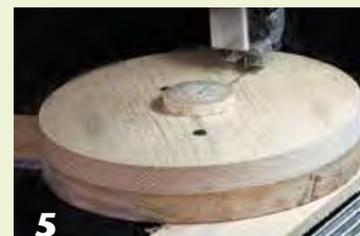
**5** Cut a slot in the disks that will house the two tree-pattern pieces. (Avoid the screws.)
