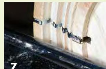
**7** Turn the inside tree profile of each disk. The black paint on the pattern warns you when to stop.
